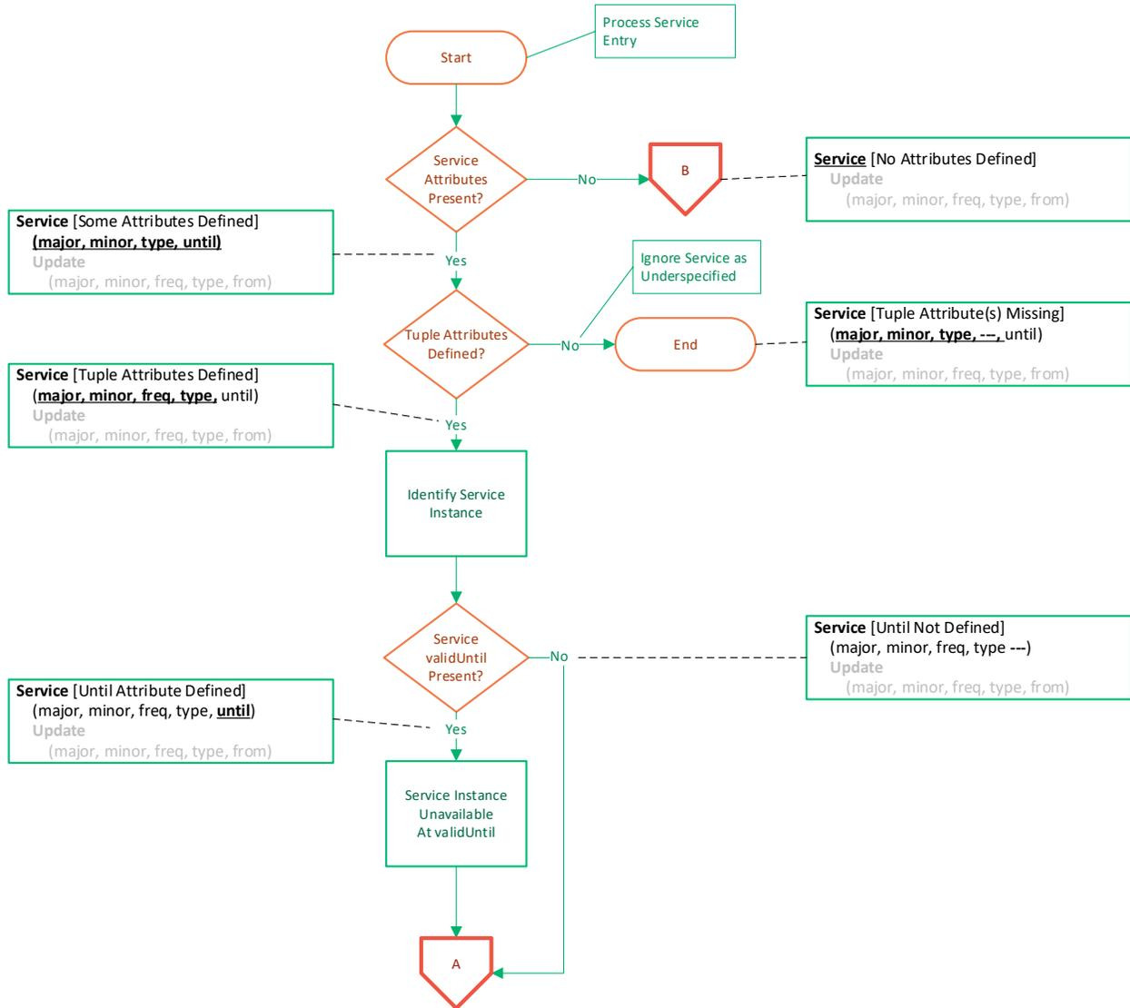
Figure A-1 RSAT Processing Flowchart – Sheet 1.
