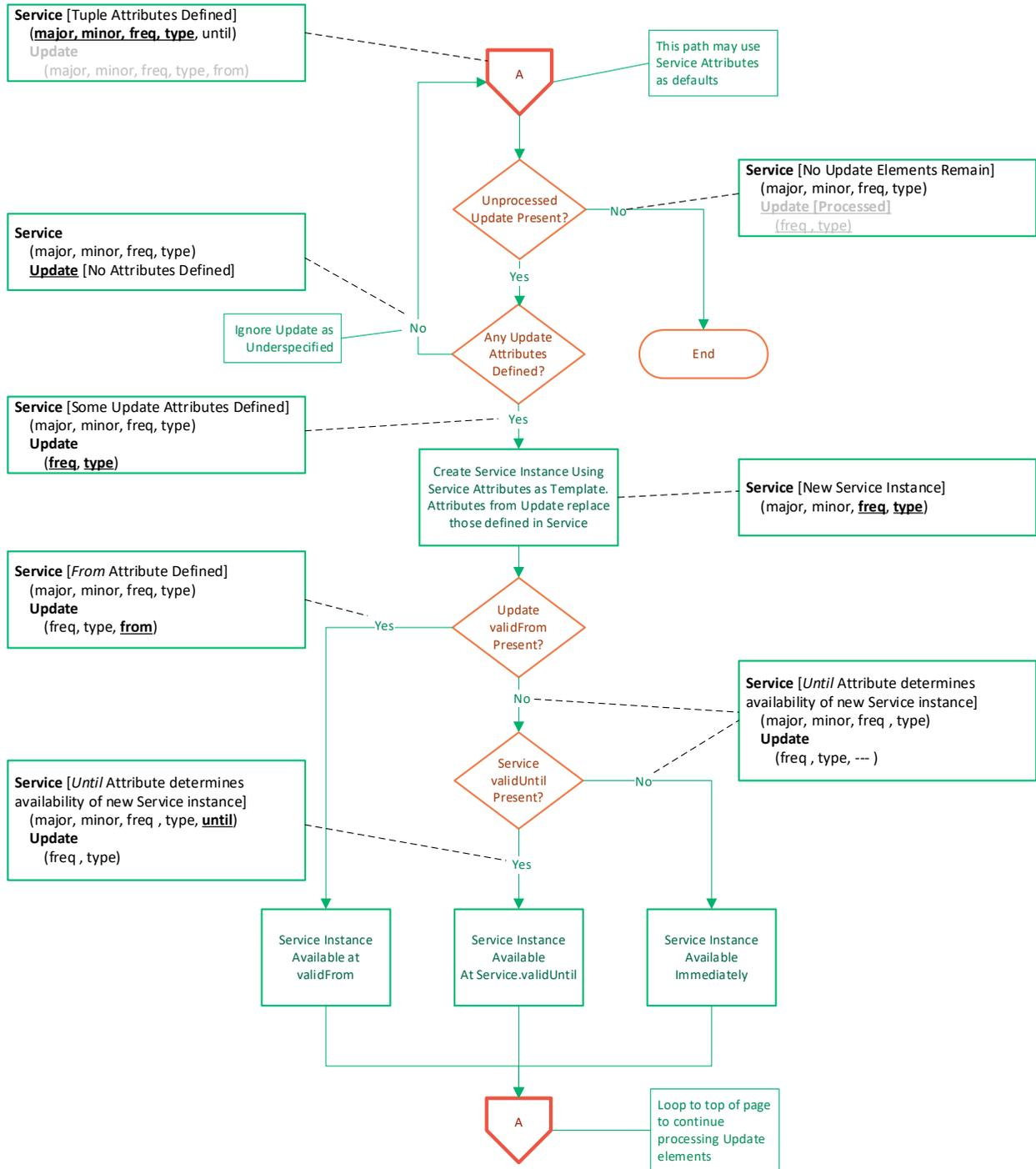
Figure A-2 RSAT Processing Flowchart – Sheet 2.
